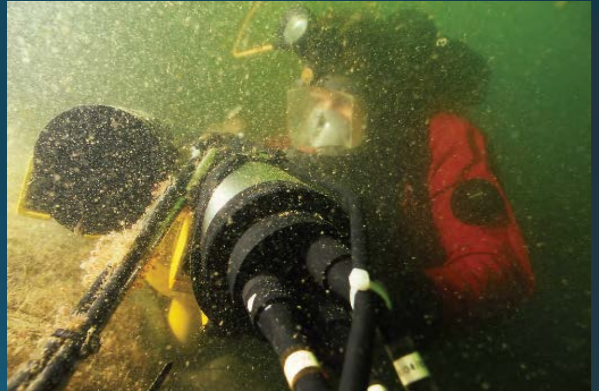
A diver with a data logger on the seabed. This apparatus measures the changes in several parameters such as salinity and dissolved oxygen. (BZN 10 wreck, the Netherlands). © R. Obst
